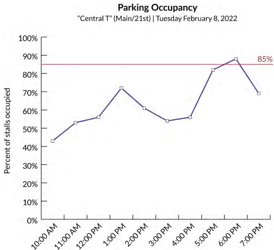
Figure 12: Percentage of stalls occupied by hour within highest demand area during weekday study day
