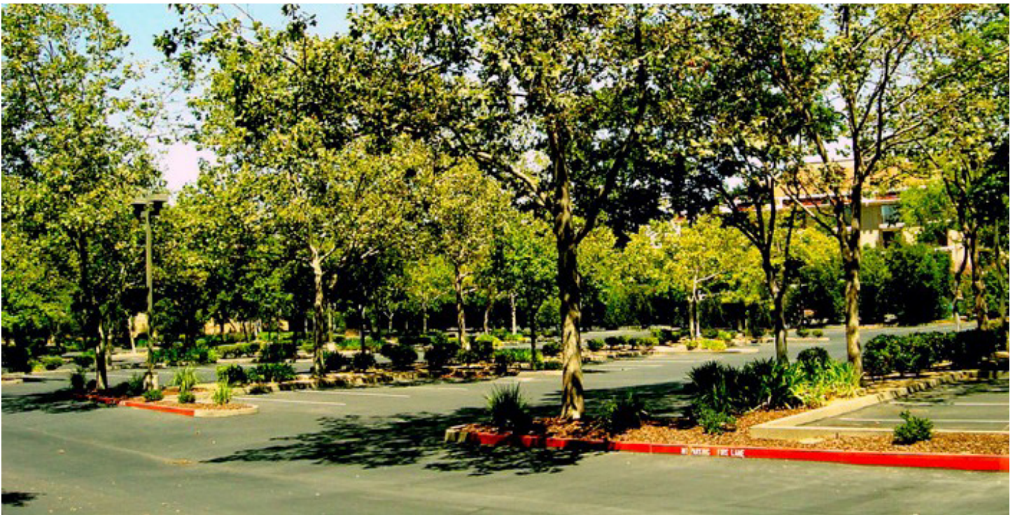
Figure VII-22: An example of using trees and plantings to manage stormwater and provide shade in a parking lot
