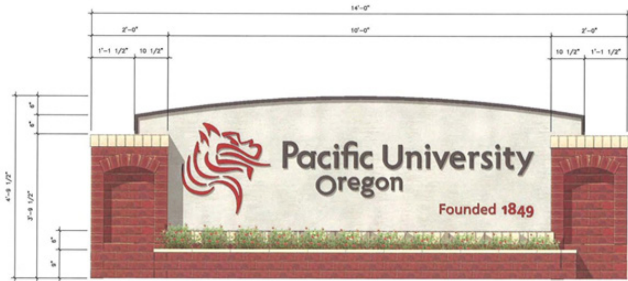
Figure VIII-2: Proposed Monument Sign with Dimensions. Main body of sign is approximately 40 SF.
