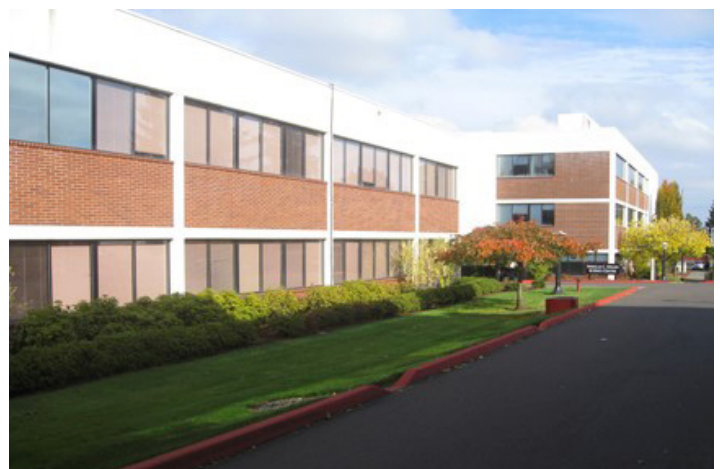
Figure VII-9: Unshaded southern building façades can lead to excessive energy use. Deciduous trees can help provide seasonal shading.
