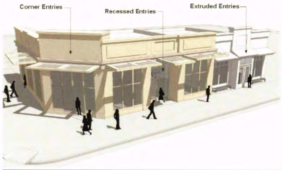
Figure 8-9 12: Example of Building Entry Design Elements
