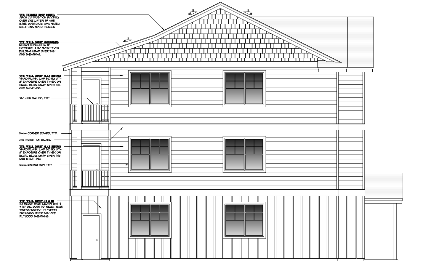
LEFT SIDE ELEVATION SCALE: 1/4"=1'-0"
