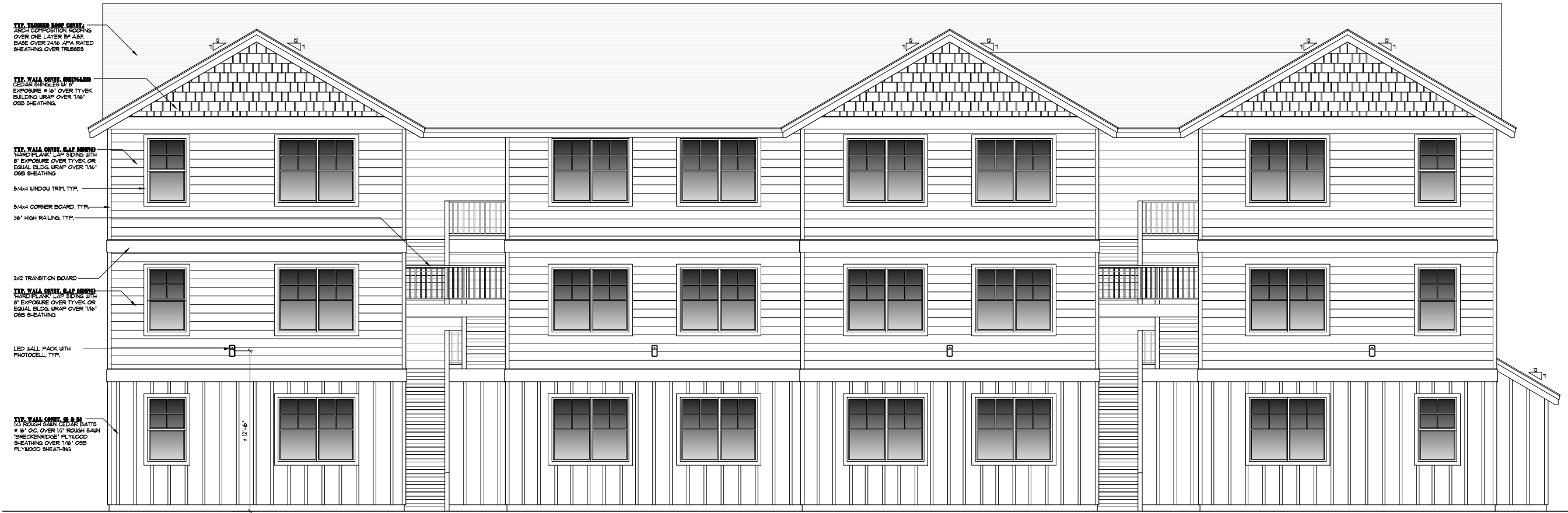
FRONT ELEVATION SCALE: 1/4"=1'-0"
