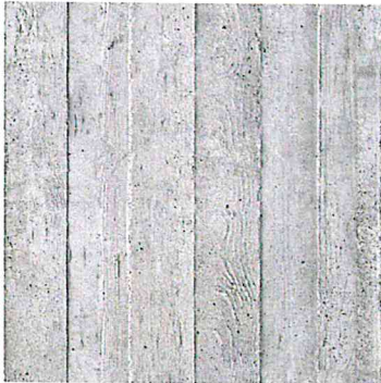
BOARD FORM CONCRETE
